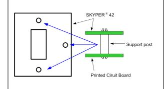
The connection between driver core and adaptor board should be mechanical reinforced by using support posts. The posts have to be spaced between driver core and adaptor board.
